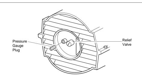
Figure 6 - Pressure Gauge Plug Removal
